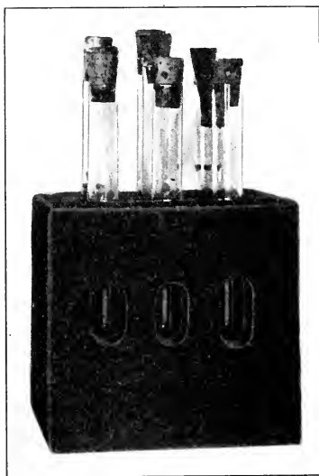
FIG. 111.—“Comparator block” for H ion determination. The three tubes in the front row contain the medium. The two behind these on the outside contain respectively the color pairs next above and next below the end point desired. The other two tubes in the middle row contain distilled water. This is a photograph of a 5-in. block.
